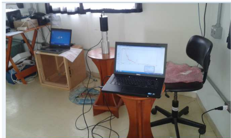
Figure 4: View of the Nai(Tl) Scintillator And PC Running the Spectrum Inside the Room with 25 Meter High in Tour on December 08, 2015
